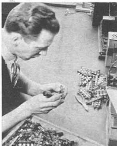
17 - INSPECTING SWITCH CONTACTS
