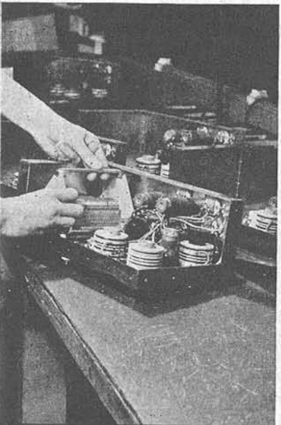
22 - FINAL OSCILLATOR ASSEMBLY
