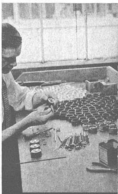
9 - ASSEMBLING SLIDE-WIRE ATTENUATORS
