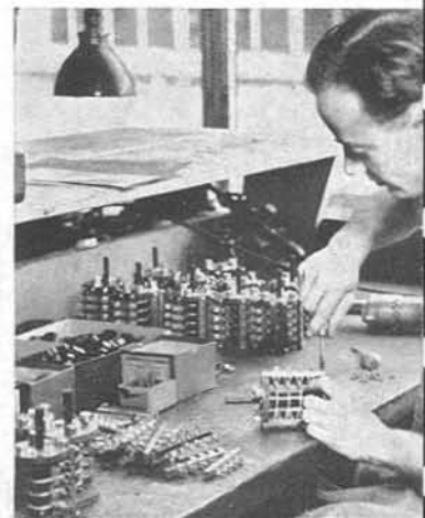
18 - ASSEMBLING FREQUENCY-CHANGE SWITCHES
