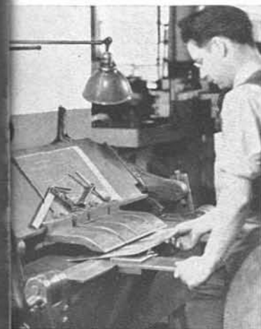
16 - FORMING OSCILLATOR SHELF ENDS
